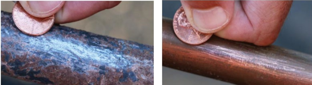
Figure 2. Scratch test on lead pipe (left) and copper pipe (right).
