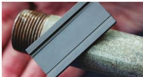
Figure 3. A magnet stuck to a galvanized steel pipe.
